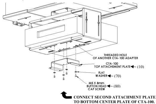
Figure 9. Install Second Attachment Plate
